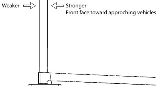
***They are a deterrent only, NOT a structural barrier. Fold-downs have NOT been designed for parking space protection and should NEVER be sold for that application.***
